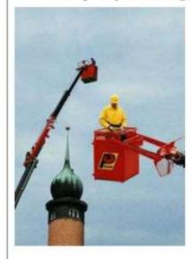
Work platforms assembled with loader cranes
