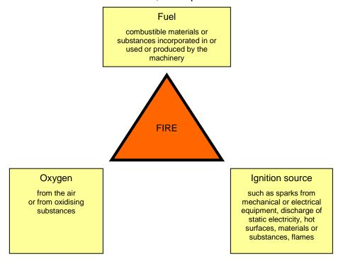
Reducing the risk of fire involves taking a combination of measures with respect to the three elements of the triangle:
